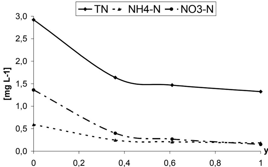
Figure 2 – Concentration profiles through the wetland. TN: total nitrogen; NH4-N: ammonium nitrogen; NO3-N: nitrate nitrogen; y: fractional distance from the inlet.
